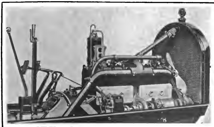
Exhaust side of the new Jeffery six engine, showing its low mounting. Note hot air connection for carburetor, drive of electric units and two-bladed aeroplane type fan
